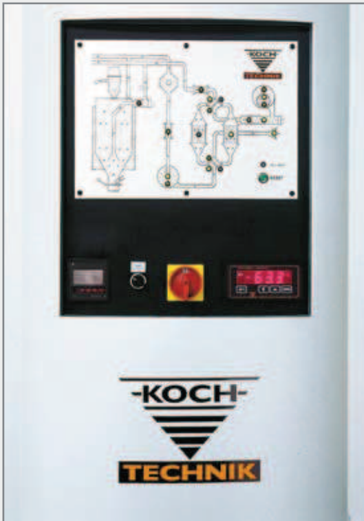
EKO standard model: A functional diagram with LEDs provides information about the operating status at all times
