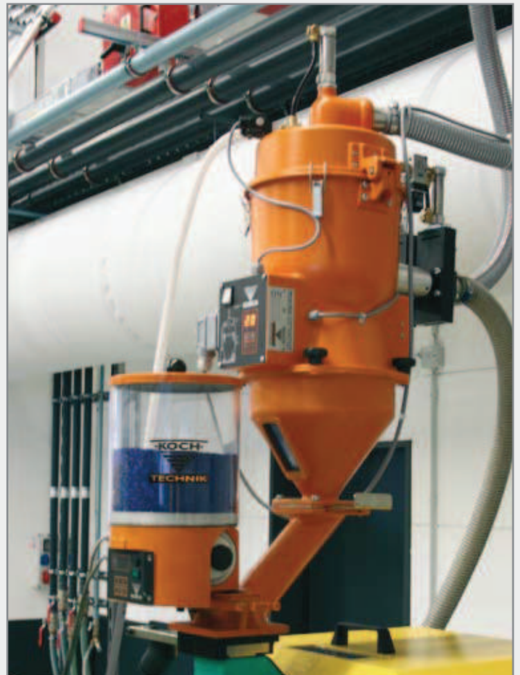
KEM, TmA 8, Z5, AZ flange: a direct colouring device with two-component-hopper loader for virgin material and regrind – processing in the central conveying system
