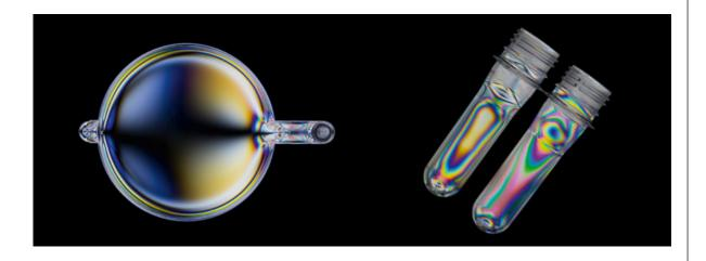
Even small internal stresses can have a negative impact on the function of optical components. Light waves which would otherwise be white can be converted into color images using crossed polarizers. The interference colors made visible this way can now be easily classified into stress ranges.
