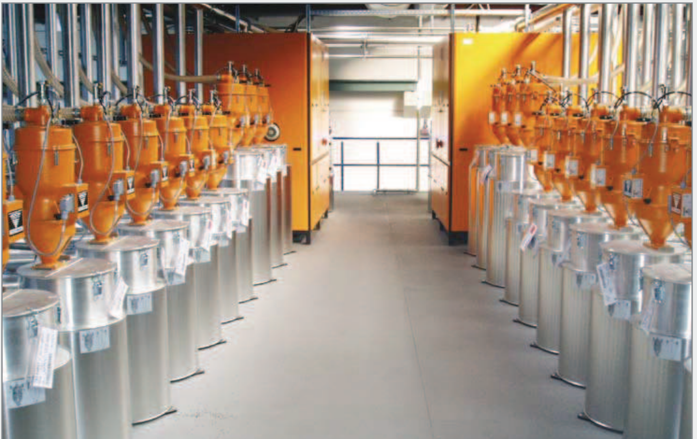
CKT 1000 dehumidified air dryers installed in the production of an automotive supplier
