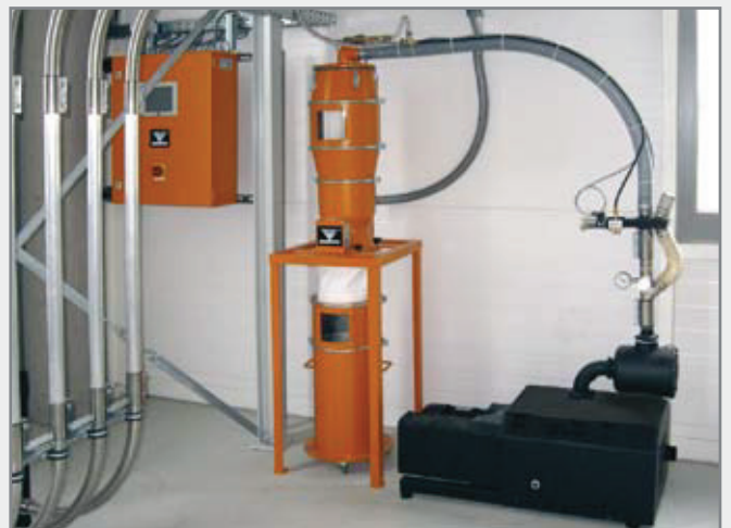
Sa 3 safety filter with PLC control unit (left) and vacuum generator
