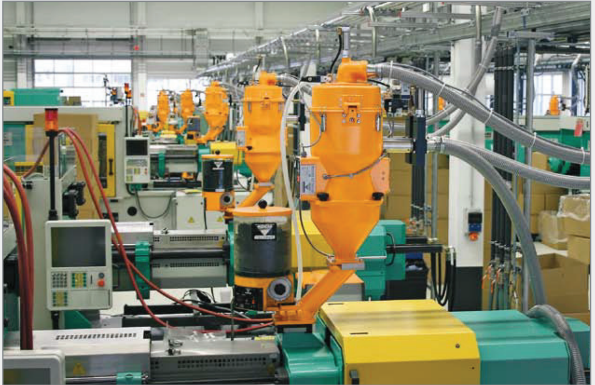
Central conveyor system with direct dyeing using a KEM / AZ / Z5 + TmA8 hopper loader.
