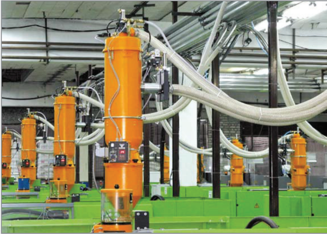
Central conveyor system with direct dyeing using a KEM / AZ / Z12 + TmA30 hopper loader.
