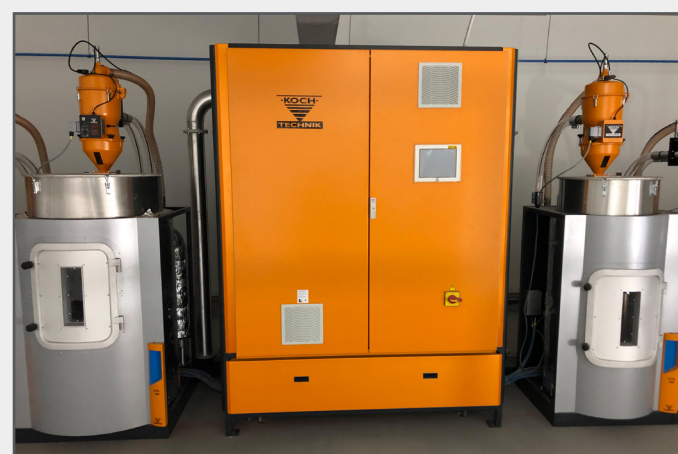
Nine different dryer sizes from EKO-N 110 to 2000 (m 3 / h) are available
