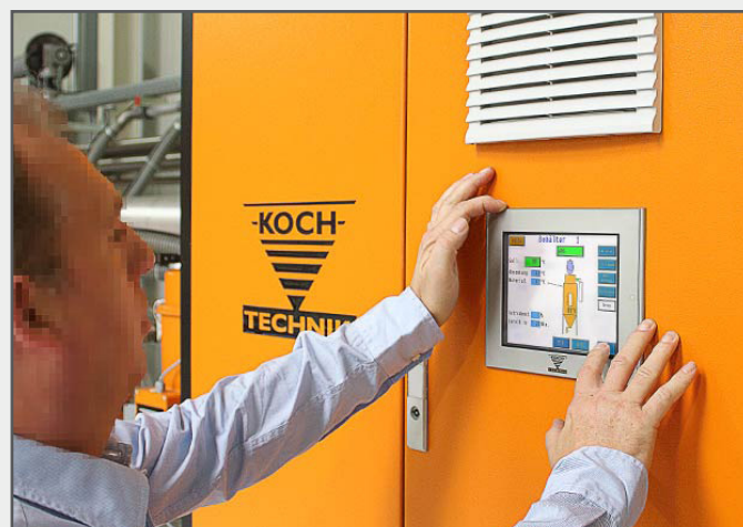
All EKO-N dryer come both with S7 control unit and a 10,4" Touch-Screen Display
