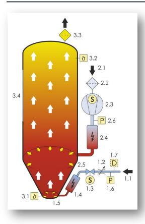
Ambient air (2.1) is drawn in by a speed-controlled blower (2.3) through an air filter (2.2), heated up in the heater (2.4) and blown into the drying hopper through the distributer ring for ambient air (2.5).
