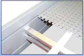
Our standard polypropylene link belt is impervious to oil, water and is able to operate with product temperature of 104°C (constant). We have nevertheless access to a wide range of belt enabling us to respond to your individual requirements. Also, stainless steel components can be fitted to the conveyor to suit a water bath application.
