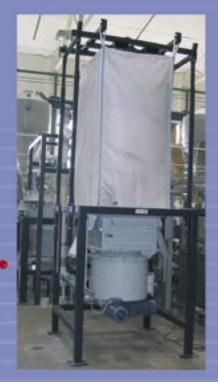
Feeder outlet type AFT, with T change over into elevating conveyor
