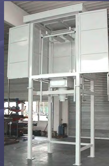
Emptying stations with housing
