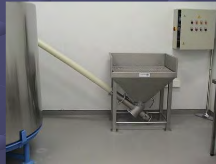
Rectangular version with grid as bag support plate and spiral conveyor
