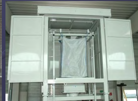
Emptying stations with housing
