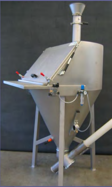
Angle of the cone depending of product to be conveyed
