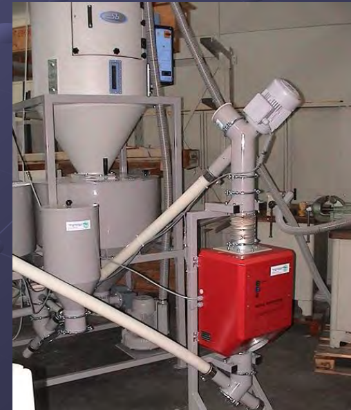
Dosing device for 3 components with interconnected all metall- separator to feed 2 blow-molding automats, hopper for new product with dryer. feeding of the hopper for mill material Straight from the mill.
