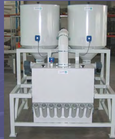
Dosing of 2 components to feed a hopper with 8 connections for pneumatic conveying
