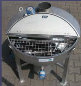
Stations with base plate, hinged lid, automatic electro-pneumatical filter cleanse and hopper to be connected with spiral conveyor Design in steel or stainless steel.
