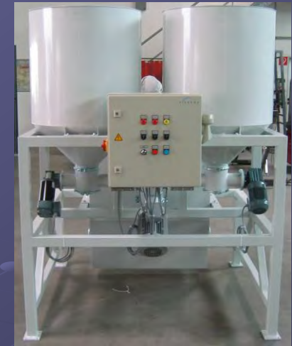
Dosing of 2 components to feed a hopper with 8 connections for pneumatic conveying
