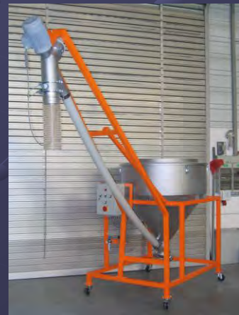
Mobile and rideable bag emptying stations with spiral conveyor
