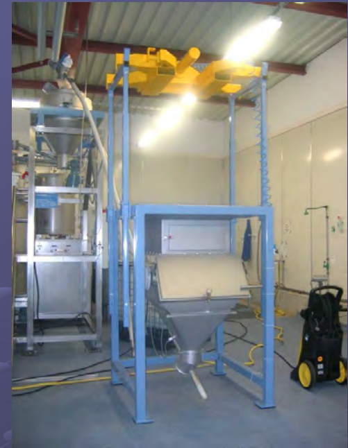
Big bag emptying with additional bag emptying hopper for good flowing products
