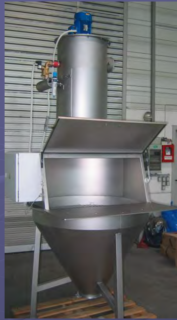
Stations with base plate, hinged lid, automatic electro-pneumatical filter cleanse and hopper to be connected with spiral conveyor Design in steel or stainless steel.
