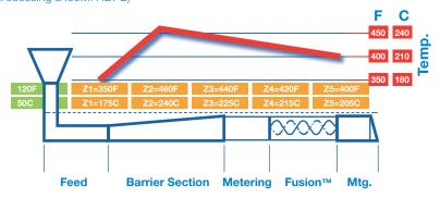
Xaloy recommends that a "hump" type barrel zone temperature profile be used to optimize the performance of the Xaloy® Fusion™ Screw. Make sure that you request the best temperature profile from your Xaloy representative for your resin and process.
