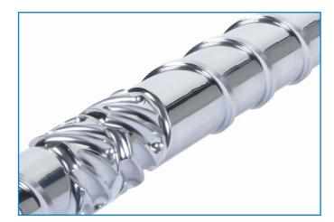
The unique, patented geometry of the Xaloy<sup>®</sup> Nano<sup>™</sup> mixer provides exponential mixing action. Its melt channels have multiple inlets and outlets that divide, reorient and recombine the melt stream.
