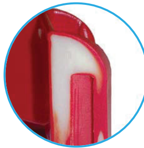
Joint for Building Construction Core: Glass-filled ABS Skin: ABS
