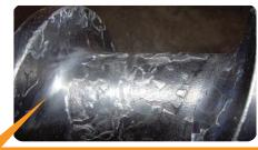
Typical poor adhesion and chipping of competitive carbide coatings
