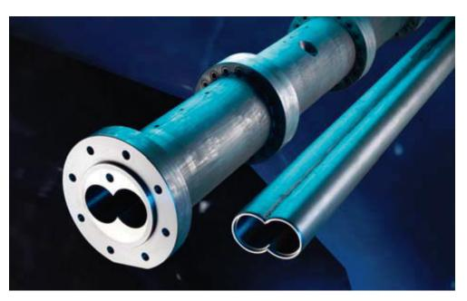
Relining job uses new liner at right as an insert for an existing bored-out casing.
