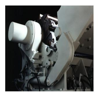
Upon request the granulator can be equipped with replaceable wear plates that are located on specific product contact areas.
