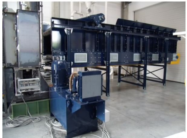
Guillotine Cutter GS 1500/1000, feed via a storage conveyor with suspended overhead pressing device; discharge via an inclined conveyor belt.
